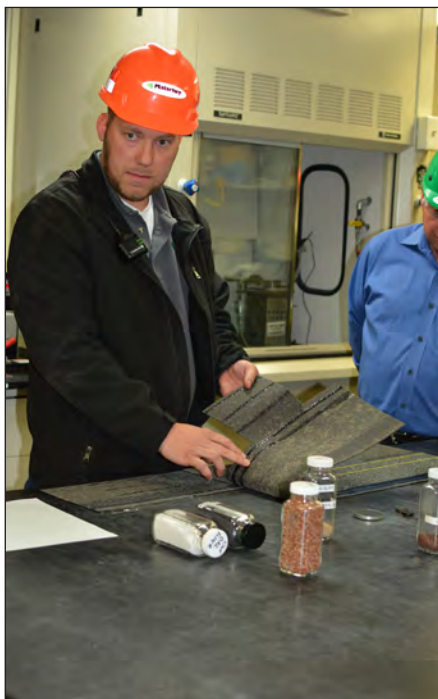
Malarkey Roofing's patented "Zone" technology includes a tapered nailing area three times larger than most other laminate shingles, which improves correct fastener placement. Improper fastener placement is the leading cause of incorrect shingle installation. Staff photo
